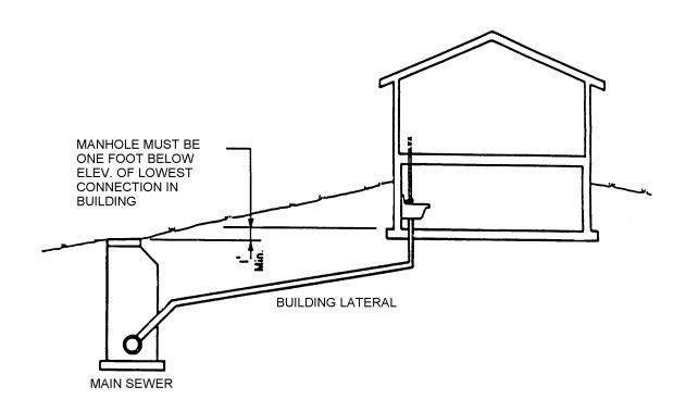
ACCEPTED DESIGN OF SANITARY SEWER HOUSE CONNECTION (SEE THE REJECTED DESIGN - FIGURE 3-1
