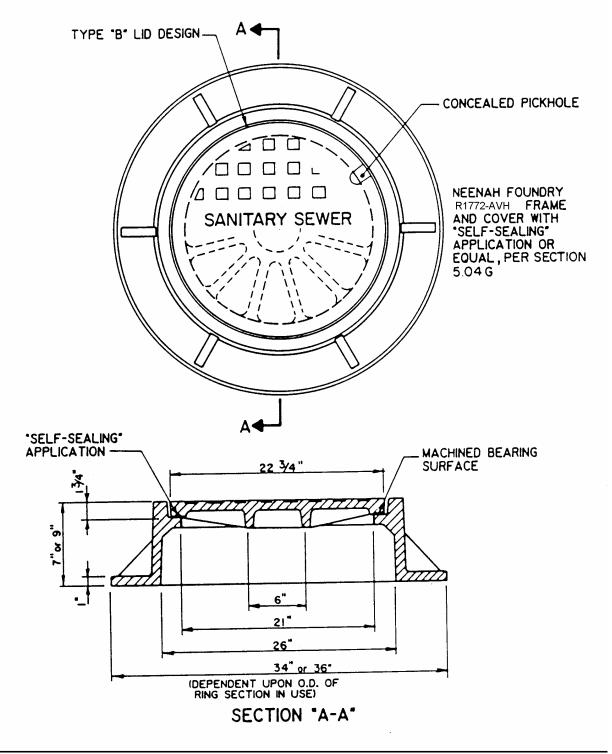
SANITARY SEWER MANHOLE FRAME & COVER - STANDARD MANHOLE
