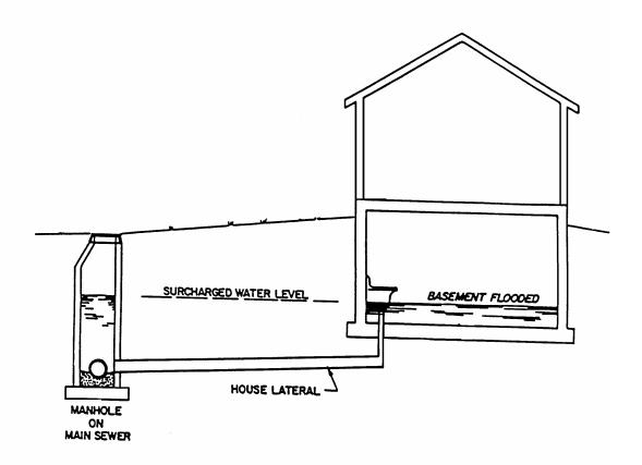
SANITARY SEWER HOUSE CONNECTION CONSTRUCTED IN THIS SITUATION WILL NOT BE ACCEPTED. (SEE THE ACCEPTED SITUATION - FIGURE 3-2)
