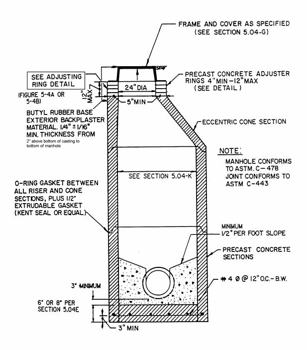
STANDARD MANHOLE FOR PIPE SIZES 8" thru 24" (Straight Thru)
