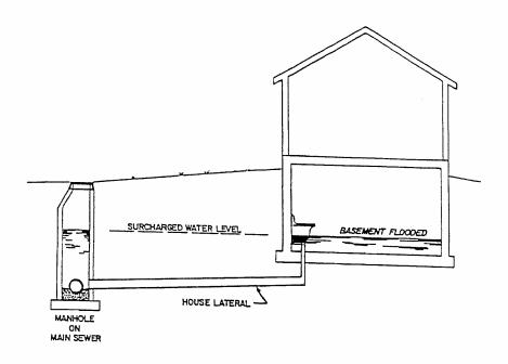
SANITARY SEWER HOUSE CONNECTION CONSTRUCTED IN THIS SITUATION WILL NOT BE ACCEPTED. (SEE THE ACCEPTED SITUATION - FIGURE 3-2)
