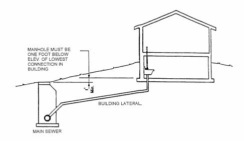
ACCEPTED DESIGN OF SANITARY SEWER HOUSE CONNECTION (SEE THE REJECTED DESIGN - FIGURE 3-1
