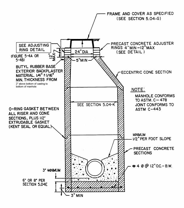
STANDARD MANHOLE FOR PIPE SIZES 8" thru 24" (Straight Thru)
